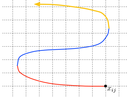
Figure 1.10: Computing an accurate approximation of the distance function to all the grid points lying on the depicted characteristic curve cannot be achieved by sweeping only once in the up-left, up-right, down-left, down-right directions: if the value T_{ij} is initialized to d(x_{ij}, \partial\Omega) , the values of T at the grid points lying on the red part of the curve are computed within a sweep of the plane in the up-left direction. Then, those on the blue part are computed using a sweep in the up-right direction. Finally, another sweep in the up-left direction is needed to compute the values of T lying on the yellow part.
