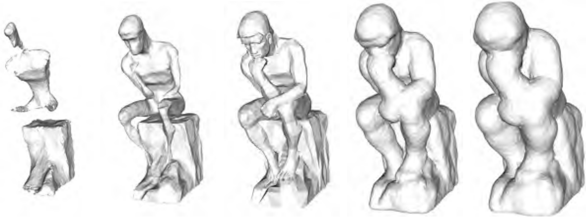
Figure 5: (From left to right): Isosurfaces -0.05, -0.02, 0, 0.03, 0.05 of the signed distance function to the (nondimensionalized) Rodin's 'Thinker' model.
