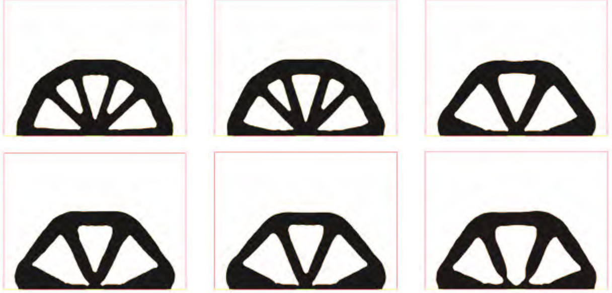
Figure 5.13: (From left to right, top to bottom): optimal shape for the worst-case optimal bridge example, for m = 0, 0.2, 0.5, 1, 1.5, 2 . The same volume constraint V = V_T = 0.75 is imposed in all six cases.
