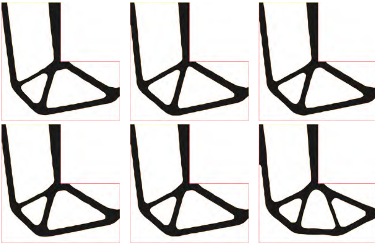
Figure 5.20: (From left to right, top to bottom): details of the test-case, optimal shape for m = 0, 0.005, 0.01, 0.015, 0.02, 0.05 , for the (worst-case) L-Beam example, using p = 2 .
