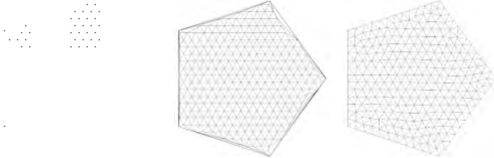
Figure 3.12: Illustration of Persson's method; (left) initial set of points \mathcal{P} , (middle) Delaunay triangulation of \text{conv}(\mathcal{P}) , and (right) final mesh after node relocations.
