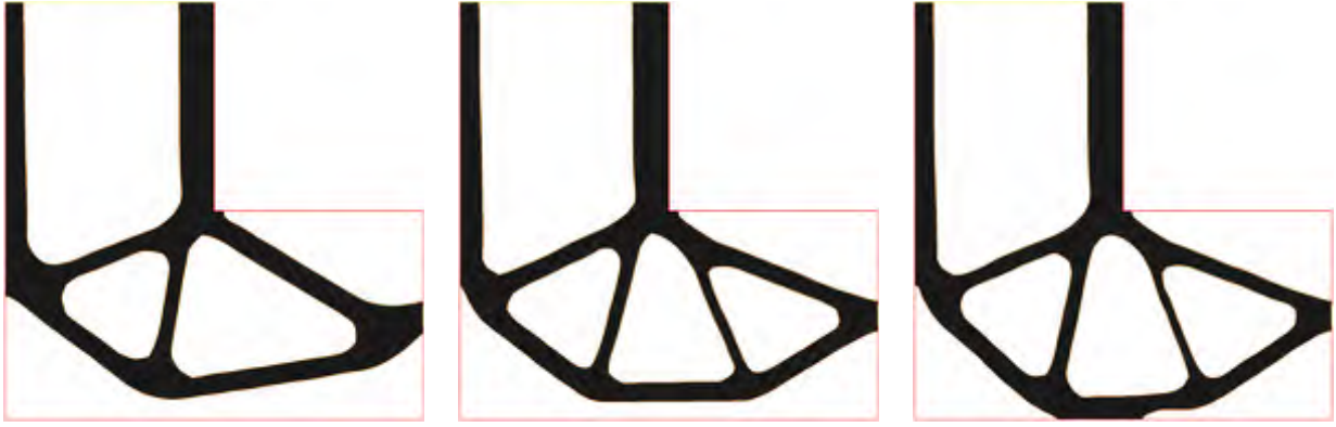
Figure 4: Optimization of an L-Beam, clamped on its upper side, subject to vertical surface loads at the middle of its right-hand side, with respect to the cost function \mathcal{C}(\Omega) = \int_{\Omega} k(x) \|\sigma(u_{\Omega})\|^5 dx , under perturbations over the geometry of the shape (see Chapter 5 for details). The same target volume is imposed on each shape. (From left to right): optimal shape for m = 0, 0.01, 0.02 .
