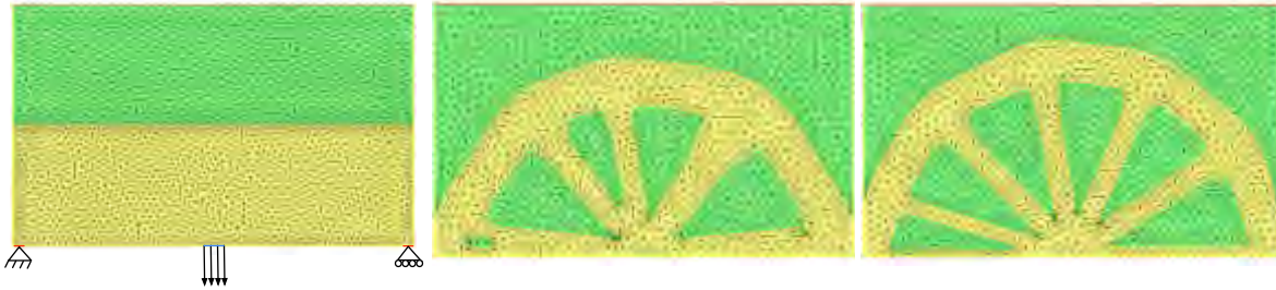
Figure 9.8: (From left to right) Initial (together with boundary conditions), 60 th and final iterations of the 2d optimal bridge test case, using information from the topological derivative.
