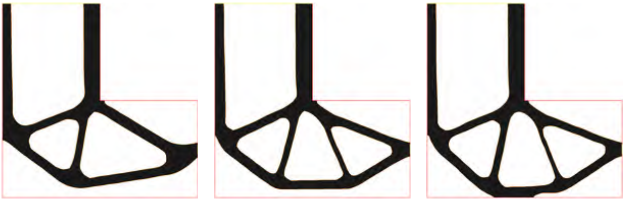
Figure 5.23: (From left to right): optimal shape for m = 0, 0.01, 0.02 , for the L-Beam example, using p = 5 .
