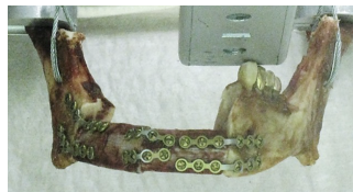
Optimization of the screws of a mandibular prosthesis [LaBa].
