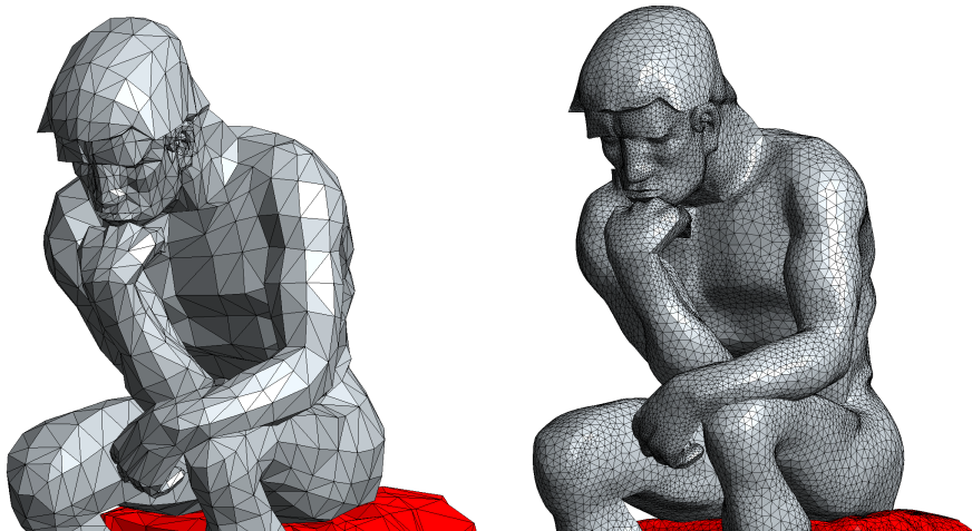
(Left) Rough approximation of a domain \Omega \subset \mathbb{R}^3 ; (right) fine geometric approximation of \Omega .
