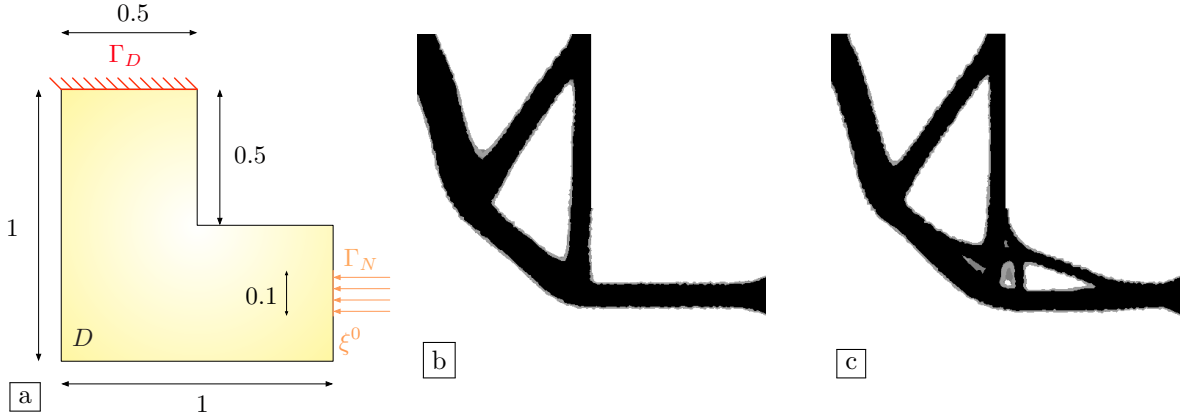
FIGURE 9. Optimal design example of an L-shaped beam considered in Section 3.4 ; (a) Setting of the test-case; (b) Optimized design h_{\text{det}}^* in the unperturbed situation; (c) Optimized design h_{\text{mean}}^* for the mean value of the compliance C(h, \xi) under the nominal law \mathbb{P} .
