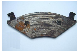
A worn out brake pad
