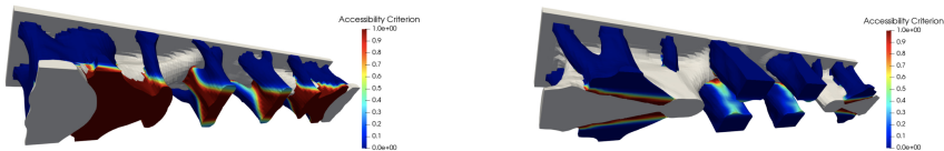
Values of the accessibility functional (Left) Without, (right) While taking into account accessibility constraints.
