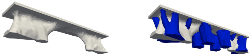
(Left) Optimized shape of the bridge \Omega (in grey) and its supporting structure S (in blue), taking into account accessibility constraints.
