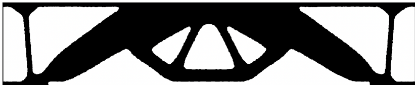
Optimized bridge under application 3 loads.
