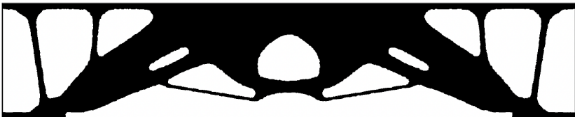
Optimized bridge under application of all 9 loads.
